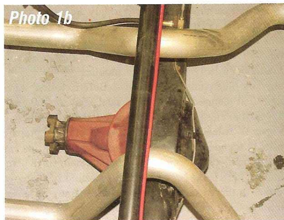
Photo #1a & 1b: The shock crossmember bolts to the rear frame rails on each side with two 3/8" x 3-3/4" bolts, washers and lock nuts on each side. The original design was a straight bar that passed right over the top of the rear end housing.
